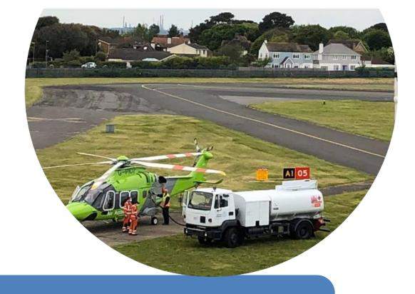
Replacement JetA1 fuel bowser subject to final sign off. This offers greater fueling capacity and faster (LPM) litre per minute supply which will encourage larger aircraft and military aircraft for rotors running refuels.
